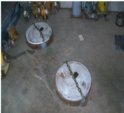
Figure G-2 Examples of source down-hole storage
