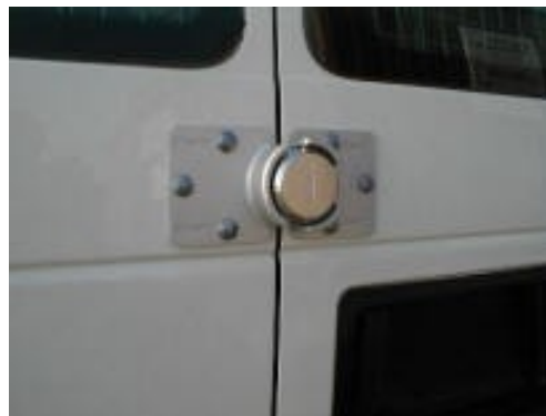
Figure 5-1 Puck lock and shield used on a cargo van
