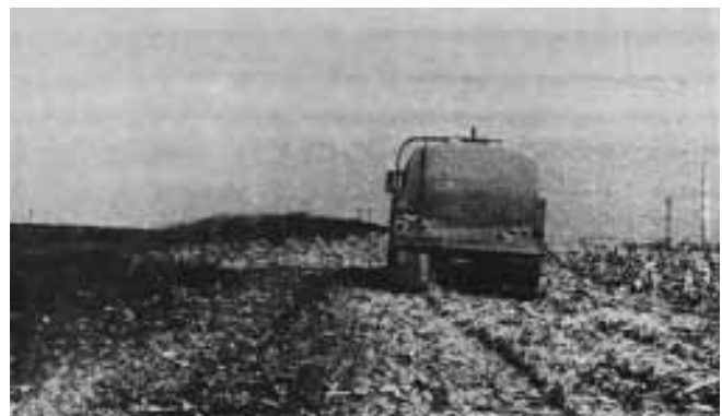
Figure 14-8. Tank truck with side spray nozzle for liquid sludge surface application (U.S. EPA, 1978).
