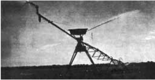
Figure 14-13. Center pivot spray application system (courtesy of Valmont Industries Inc.).
